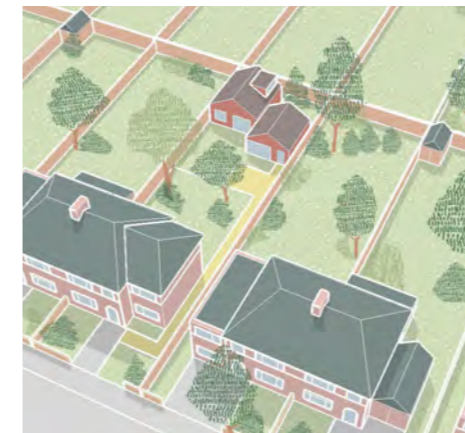
Figure 2.4.9c and 2.4.9d: Rear garden with development built along boundary and view from neighbouring kitchen window. No windows face onto neighbouring garden and proposal drops down towards boundary, to minimise loss of amenity and ensure development potential on neighbouring garden.
