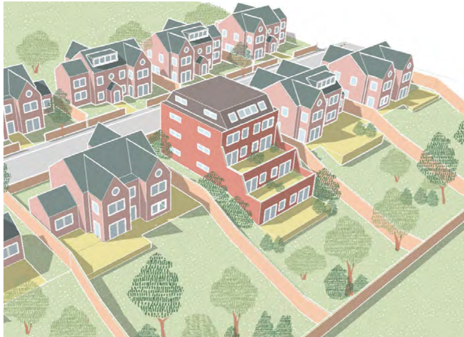
Figure 2.4.12a: Stepping massing down a hill to gain additional accommodation
