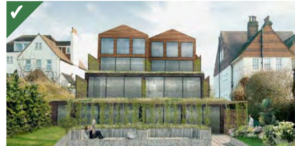
Figure 2.4.11c: Projecting flat roofs successfully used as balconies.
