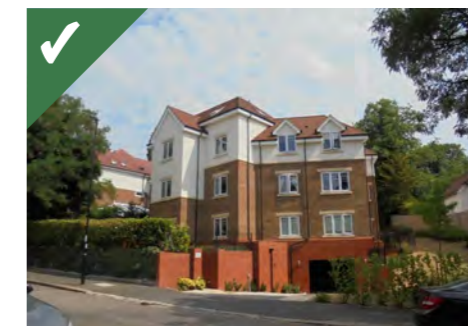
Figure 2.4.12f: Successful use of topography to integrate parking into a basement. Once matured, planting will reduce appearance of retaining wall.
