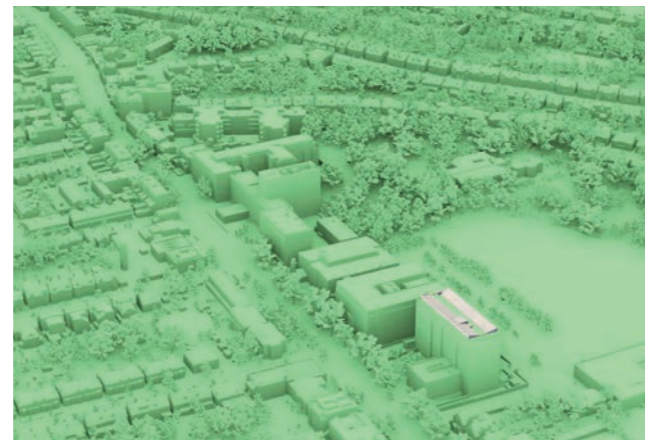
Fig 174 View demonstrating the Upper threshold with green datum line set at approximately 33m, equivalent to 10 storeys
