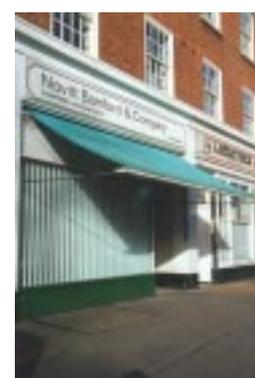
**fig. 13. Non retractable plastic blinds are not appropriate as they permanently obscure parts of the shopfront and introduce discordant materials and shapes into the street scene, particularly in historic areas**
