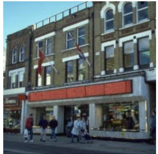
**fig. 2. The vertical division between these buildings has been visually destroyed by this shopfront**
