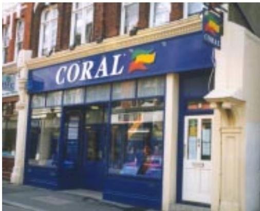
**fig. 4. Obscure glass has been used here to fill the gap between the ceiling and the bottom of the fascia**
