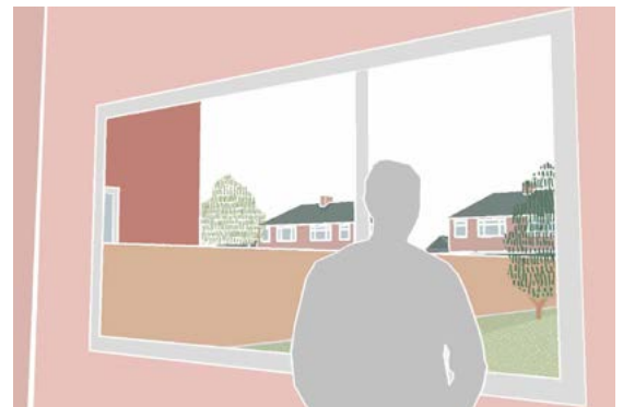
Figure 2.11i: Apparent depth of Proposal 1 limited by 45° rule.
