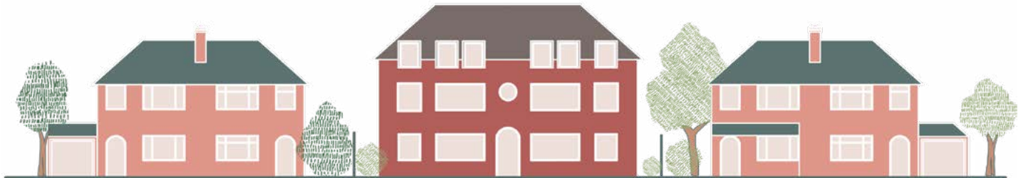
Figure 2.10e: Where surrounding buildings are semi-detached homes in a planned estate, new developments should seek to accommodate a full third storey partially contained within the roof space to ensure the characteristic scale of the buildings along the street is maintained.
