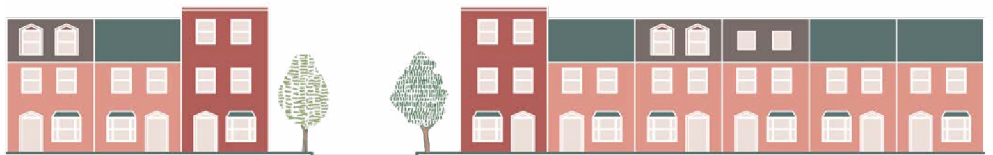
Figure 2.10f: The addition of a third storey within terraced houses will generally only be through accommodation within the roof. The acceptability of this will be based on the merit of design and the impact on street scene, given the consistent nature of continuous eaves and roof heights. A terraced house on a corner plot may seek to provide a additional full storey.
