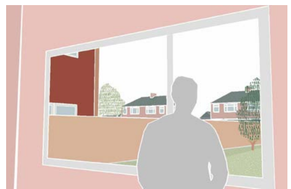
Figure 2.11q: Apparent depth of Proposal 3 limited by 45° rule.
