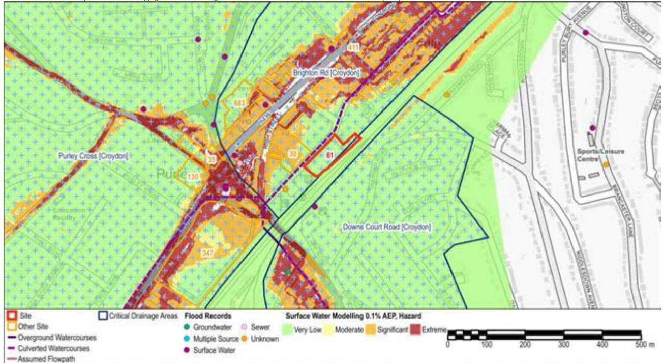
**Figure 10 - Surface Water Modelling 0.1% AEP Flood Hazard**
