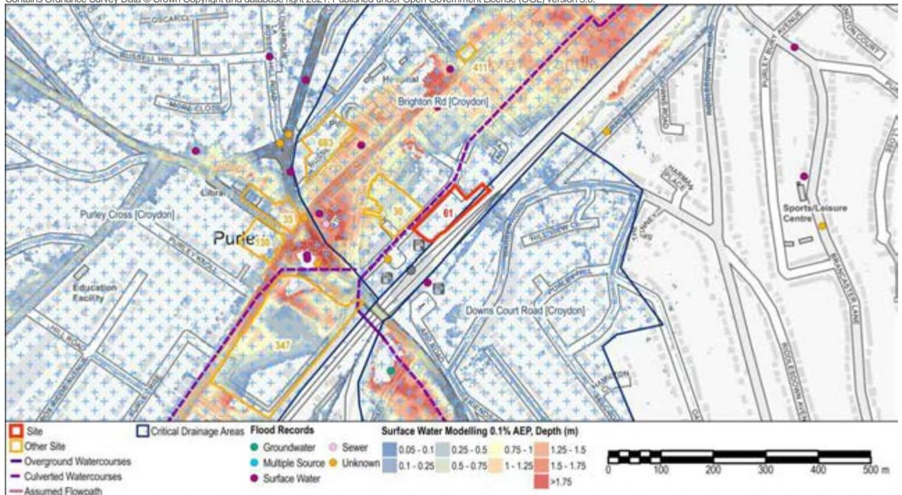
**Figure 9 - Surface Water Modelling 0.1% AEP Flood Depth**
