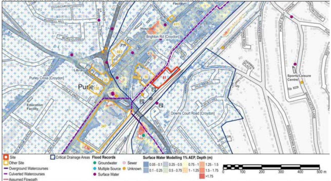
**Figure 7 - Surface Water Modelling 1% AEP Flood Depth**
