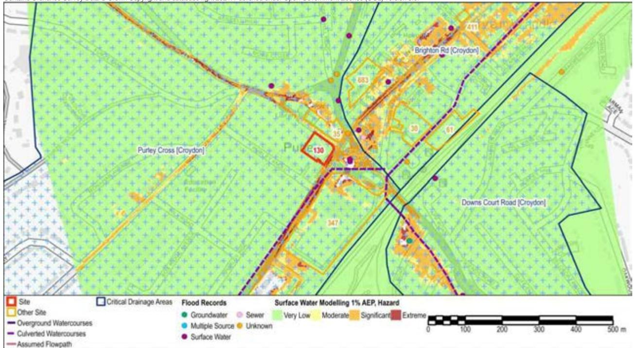
**Figure 8 - Surface Water Modelling 1% AEP Flood Hazard**
