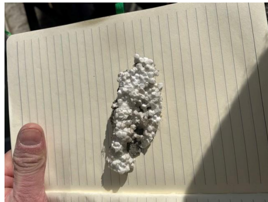
Figure 19. Location 1.3 EPS from behind the infill panel
