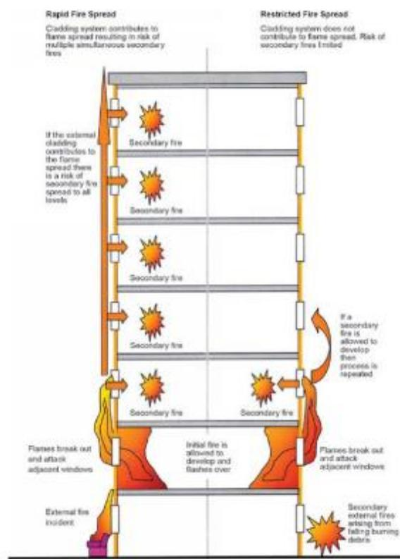
**Figure 10.** Mechanism for fire spread
