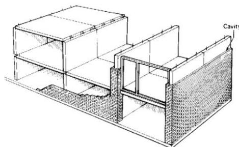
**Figure 7.** Typical brick on RC downstand
