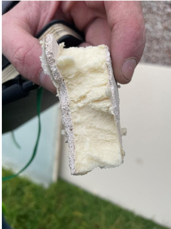
Figure 26. Location 2.1 thermo plastic insulation material
